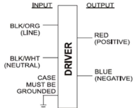
Input and output use lead-wires.
